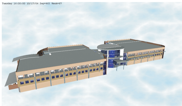
Figure 7: The Figure shows a screenshot of the construction sequencing of the Camino Medical Group project. The exterior construction is completed and interior construction is now in progress
