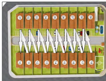
Figure 1: Construction site plan and sequence of execution
