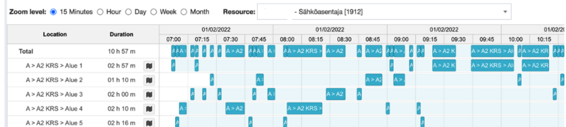
Figure 1. The figure shows an Electrician’s presence on the second floor takt areas during a working day.
