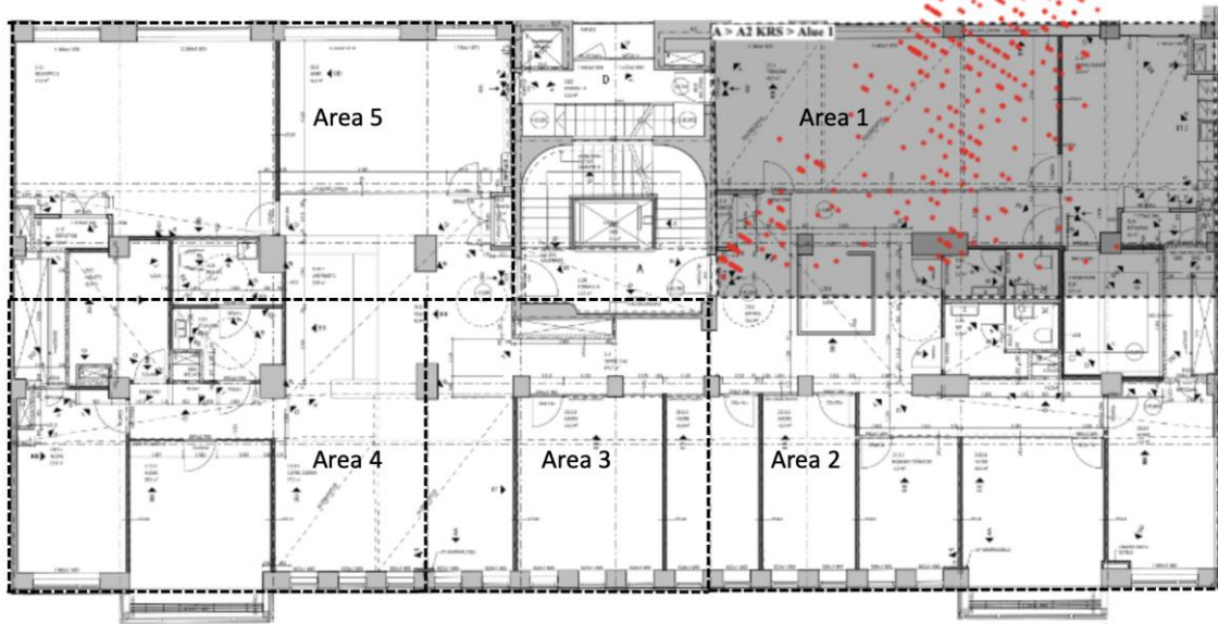
Figure 2. The figure shows an electrician’s presence indicated as red dots on the second floor takt area 1 (Alue1) during a working day.
