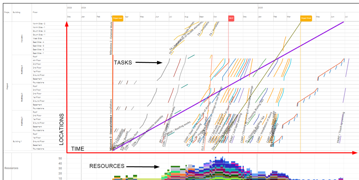
Figure 1: Location-based Schedule for Case Study A. The extra purple task from start to end has been added for extracting general site resources.
