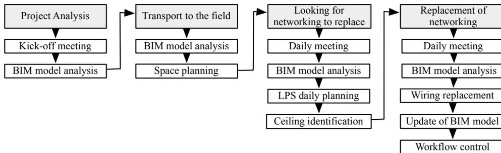
Figure 4 –Flowchart of the implemented processes
