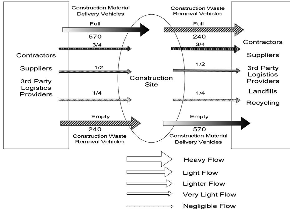
Figure 3: Integrated materials delivery and waste removal logistics
