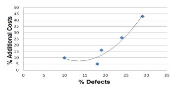
Figure 9: Nexus between the percentage of defects and major additional costs
