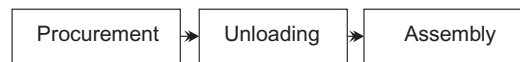
Figure 2: Flow diagram of the rebar management system used in the case study in the case of off-site fabrication
