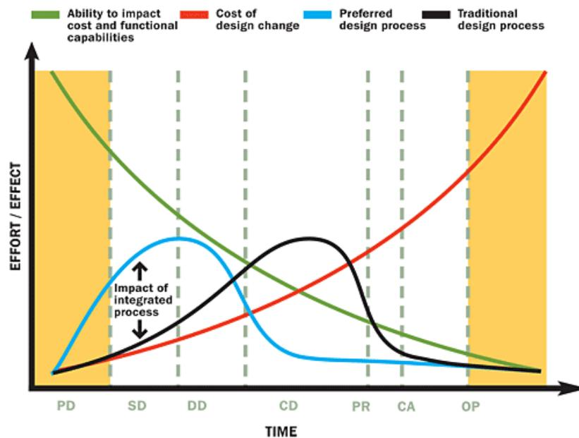
Figure 2: Preferred design process versus traditional design process (Pressman, 2007).
