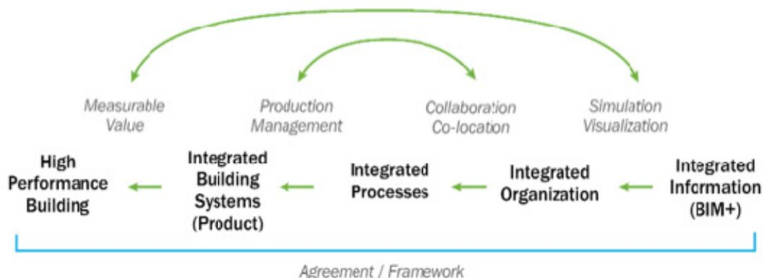
Figure 1: How integration of product, process, organization, and information supports the creation of a high-performance building (Fischer et al., 2012).
