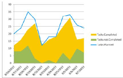
Figure 3: Committed Tasks on Plan (TOP), total tasks completed, and total tasks not completed (variation indicator)
