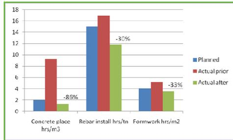
Figure 1: Unit production rate comparison within a project (planned, before, and after lean implementation)
