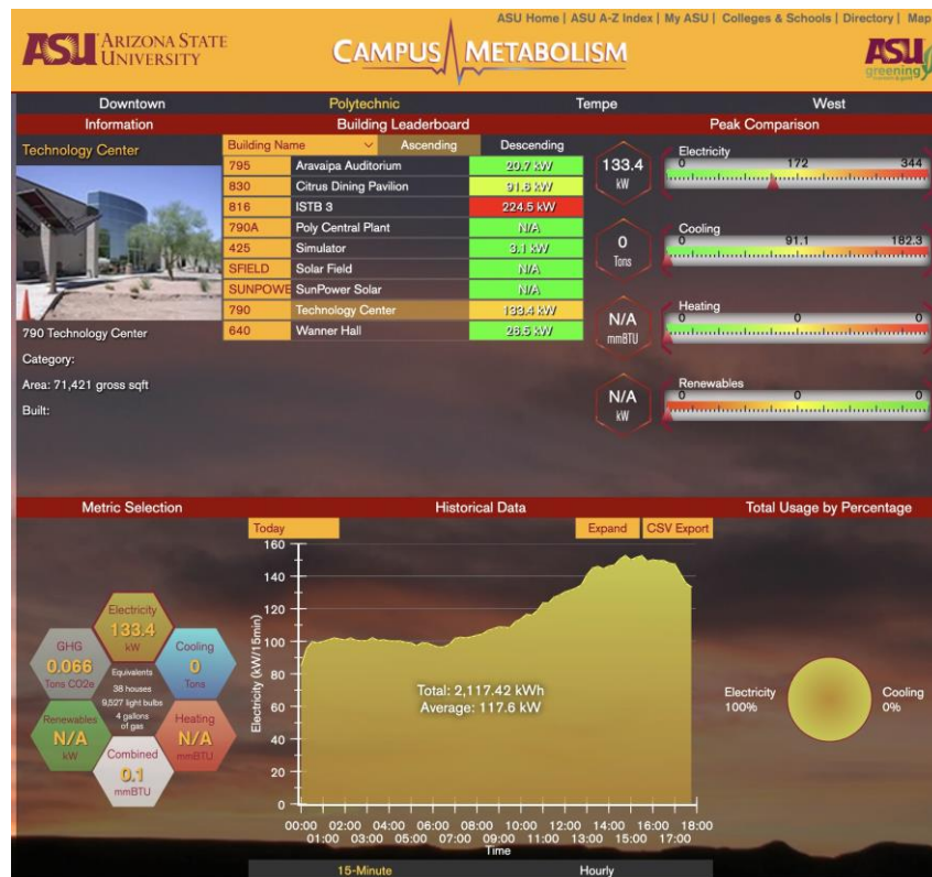
Figure 2: ASU's Energy Information System, Campus Metabolism, helps to identify buildings that may be good candidates for DR (screenshot from K. Parrish on 17 April 2024)
