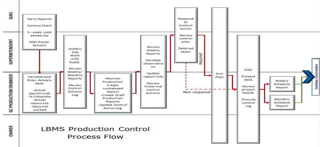
Figure 2: The LBMS process flow for production control on the hospital project
