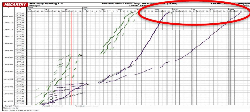
Figure 6: The flowline on 12/2012 showing 3.5 months delay in welding completion based on current production rates
