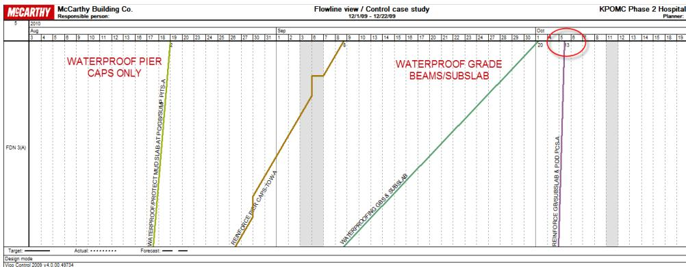
Figure 4: The additional waterproofing activity for grade beam/sub-slab between reinforcing for pier caps and reinforcing for grade beams/sub-slab
