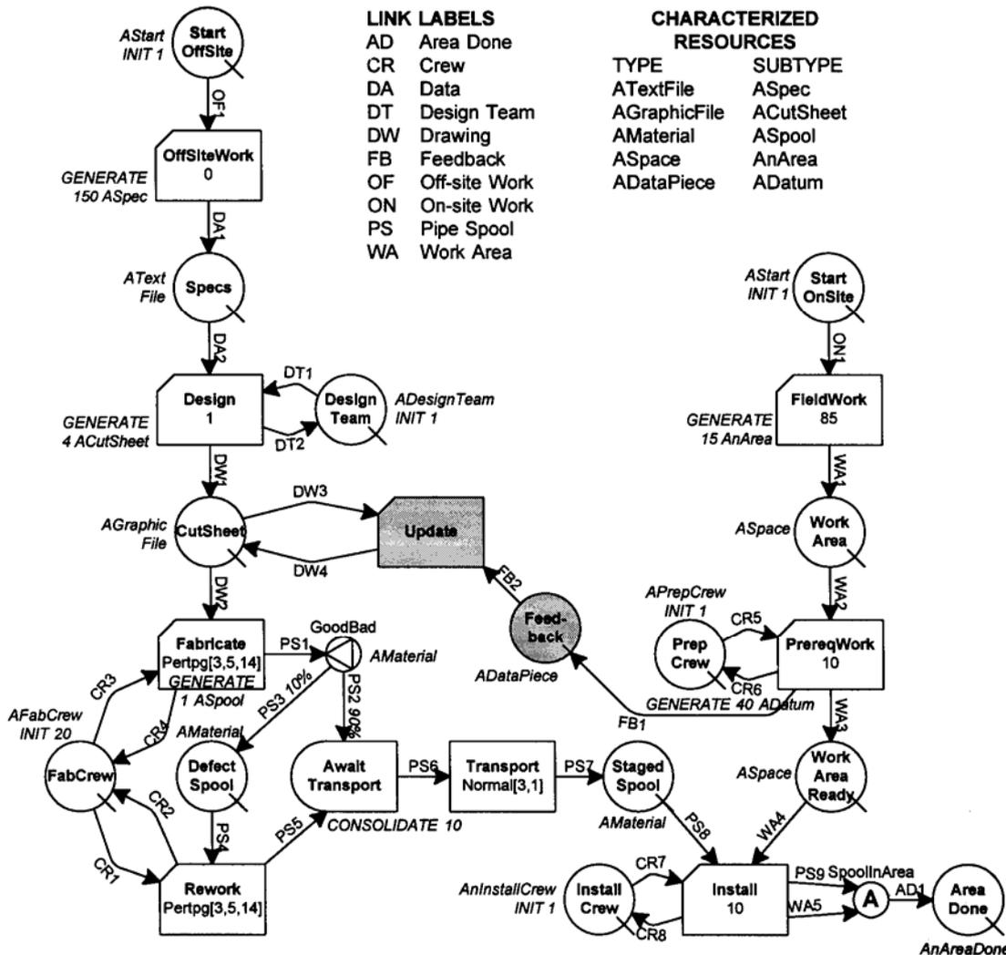
**Figure 1** Pipe-spool process model.
