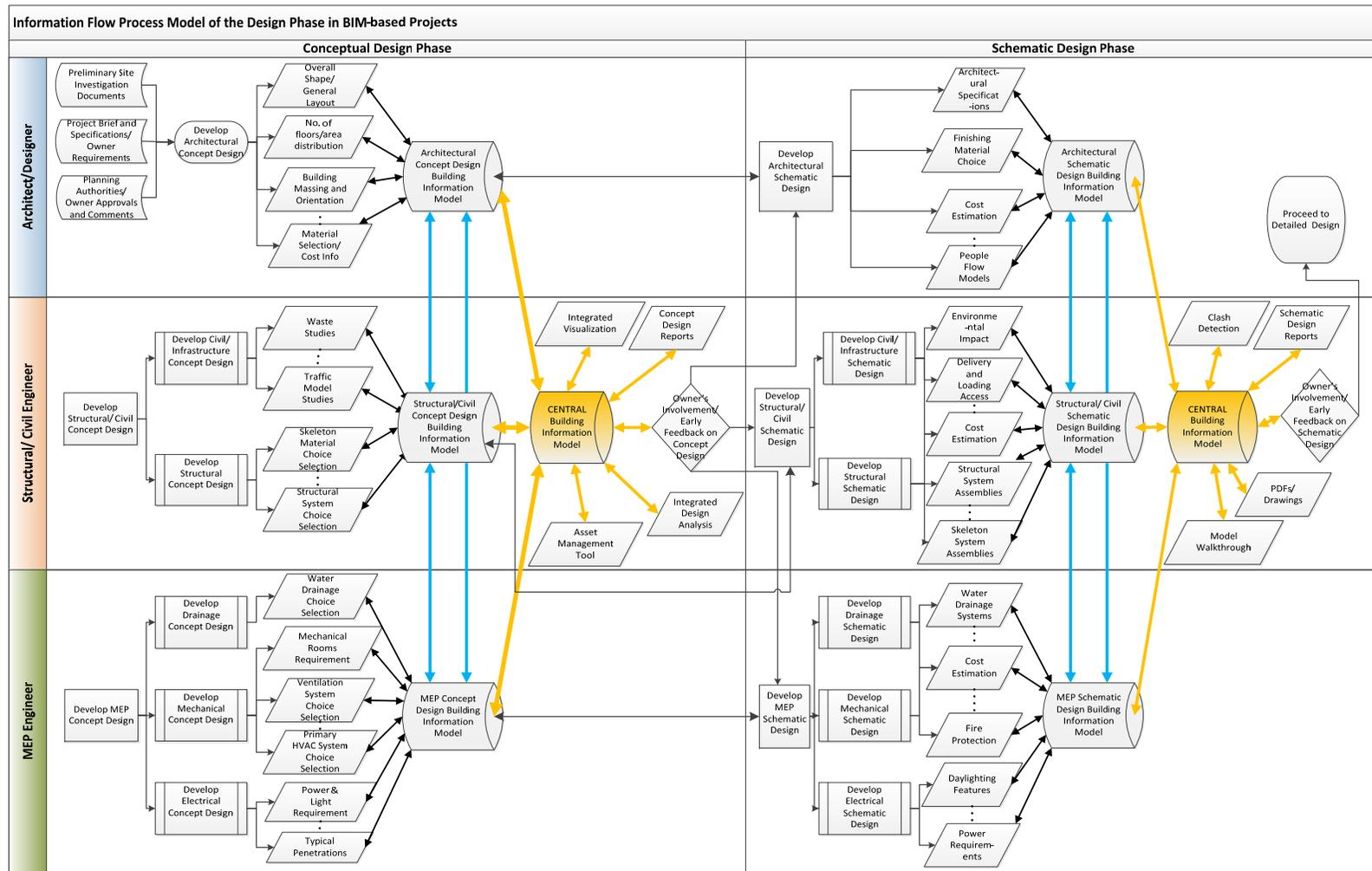
Figure 3: Information Flow Process Model of the Design Phase in BIM-based Projects
