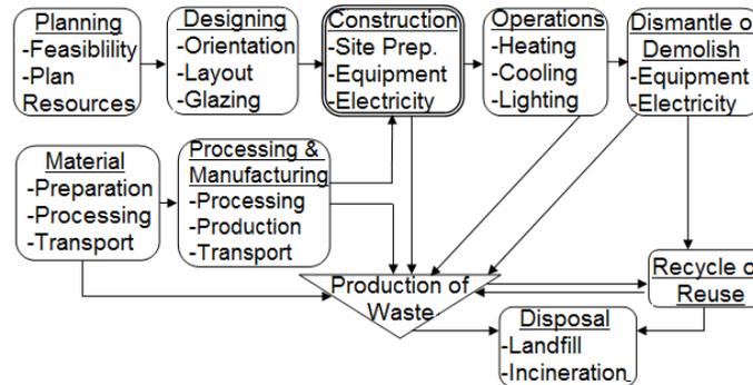
Figure 1: Typical Supply Chain Model of U.S. Construction Industry
