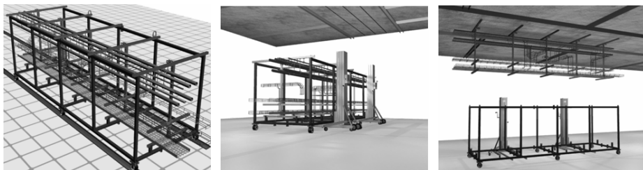
Figure 3: ATIF ready in manufacturing centre; onsite ready for elevation using mechanical lifting hoists; corridor module installed with ATIF to be returned to manufacturing centre for re-use.
