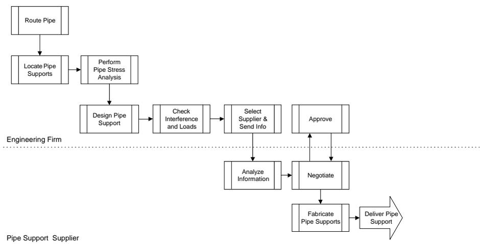
*Figure 1: Supply-Chain Configuration 1 of Pipe Supports (also see configuration 1 compared to others in Arbulu and Tommelein 2002 and in Tommelein and Arbulu 2002)*
