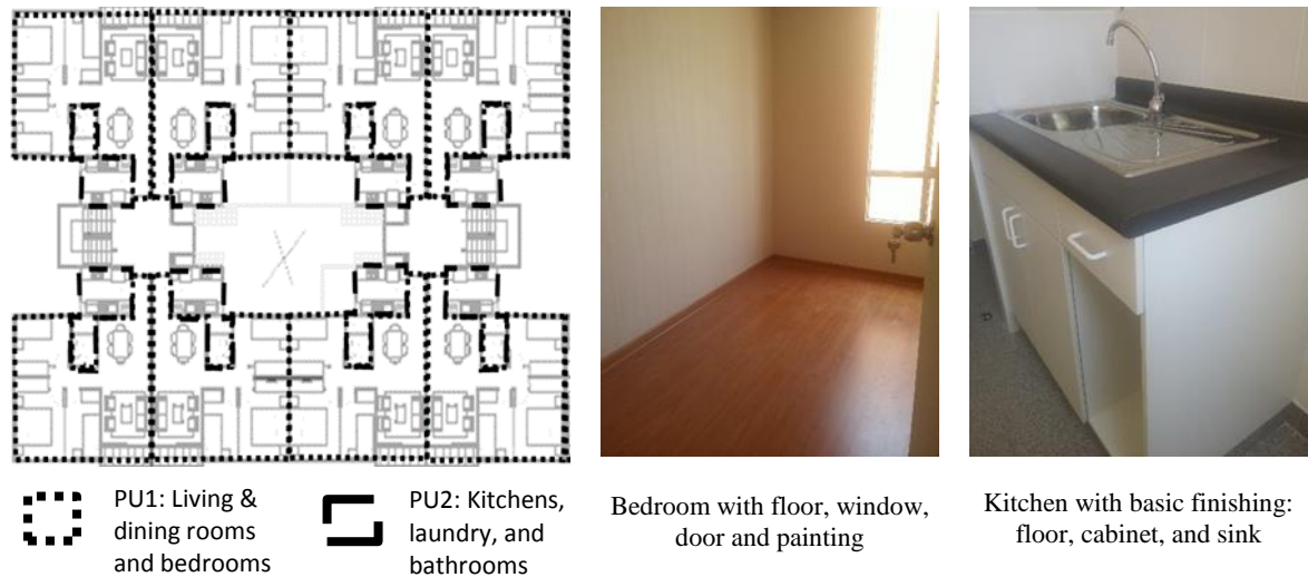
Figure 3: General plan divided into two production units
