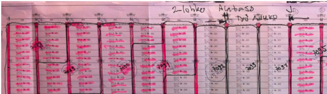
Figure 1: Image of how the actual installation schedule of precast concrete is documented and managed in Toriparkki construction project.
