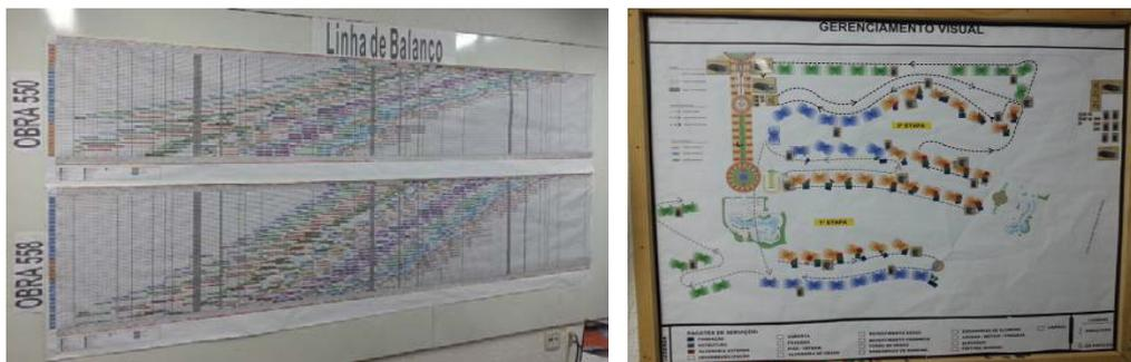
Figure 3: Line of Balance and magnetic board
