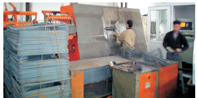
Figure 6: Computer integrated machines used by rebar fabricators
