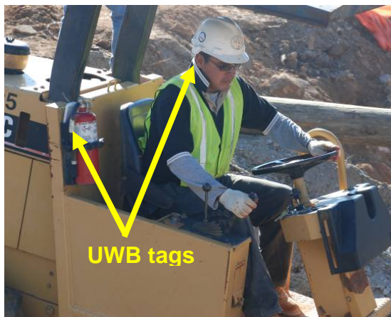
Figure 5: UWB Tags Attached to Personnel and Construction Machinery.
