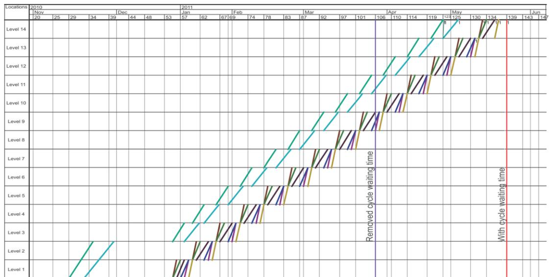
Figure 2: Apartment building planned as one pour per floor. Final Pour on Day 136
