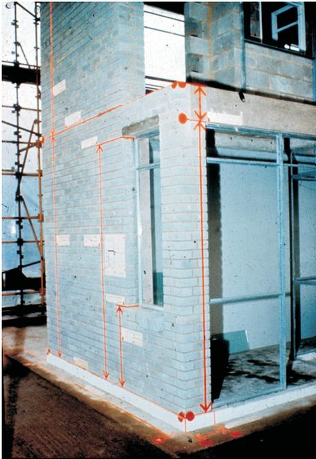
Figure 4: Dimensional control lines on the Method of Building Rig showing components within their own 'basic' space.
