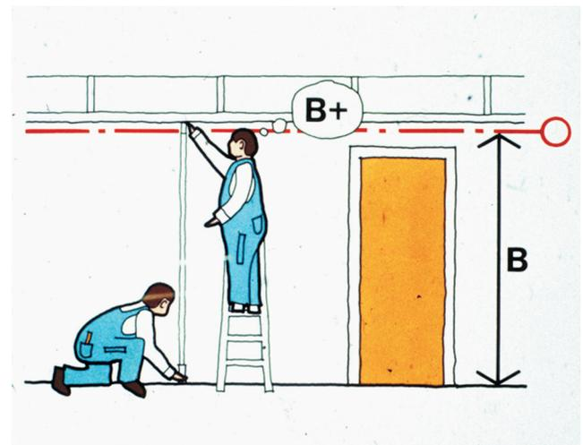
Figure.5: Tolerances in Construction meant that components sometimes lay outside their own 'basic' space.
