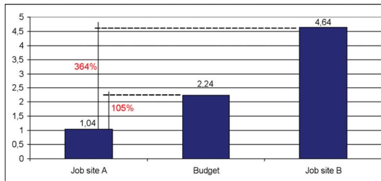
Figure 5. Crane productivity comparison
