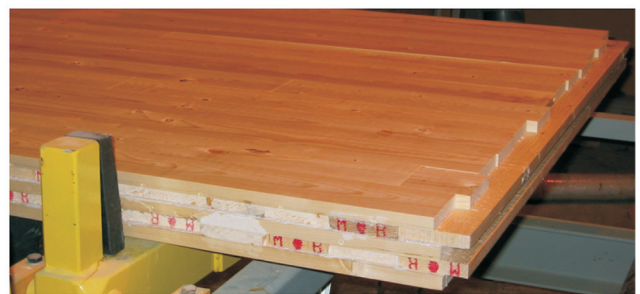
Figure 4: Cross-laminated massive timber slab.
