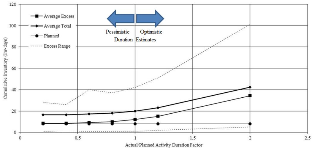
Figure 7: Cumulative Inventory Levels Versus Actual/Planned Duration Factor for Network Simulation Shown in Figure 6
