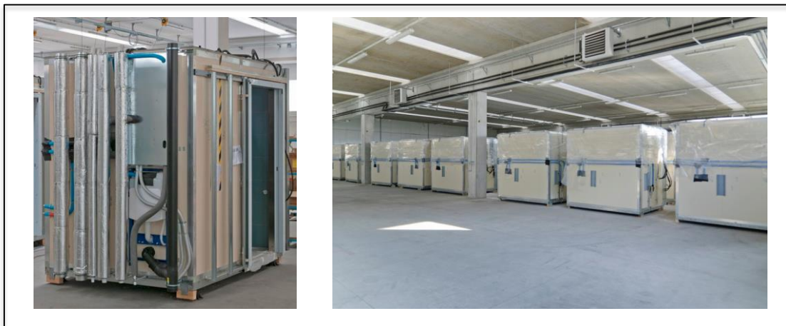
Figure 1: Example of prefabricated plumbing cells and stationary production in a hall (Sanika GmbH, Via Primo Maggio 22, 38089 Storo (TN), Italy)
