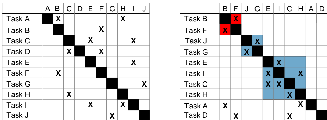
Figure 4. Example of DSM Analysis before (left) and after (right) Partitioning
