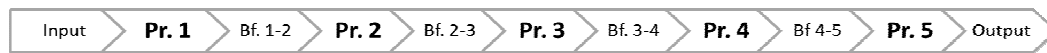
Figure 1: Simplified model of an RBP consisting of 5 sequentially dependent processes (Pr. #) and the 4 intermediary WIP buffers (Bf. #-#) (adapted from Gonzalez et al. 2009).
