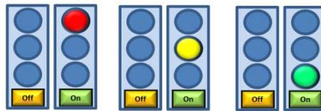
Figure 3: Traffic lights with Boolean switches. When switched on, the possible signs are red=“unsound – action needed”; yellow=“action soon needed”; or green=“sound”
