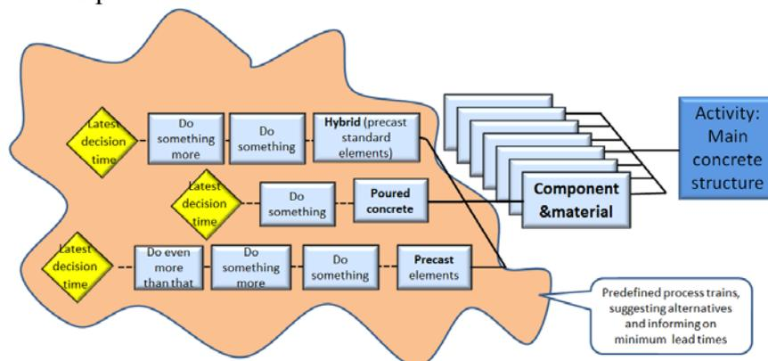
Figure 6: Using predefined process trains suggesting alternatives and specifying minimum lead times
