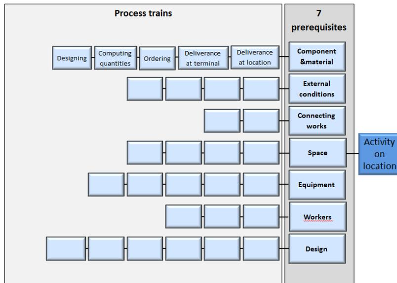
Figure 2: “Process trains” (each activity has process sequences, sets of actions, which must be completed in order for each of the seven prerequisites to be sound)
