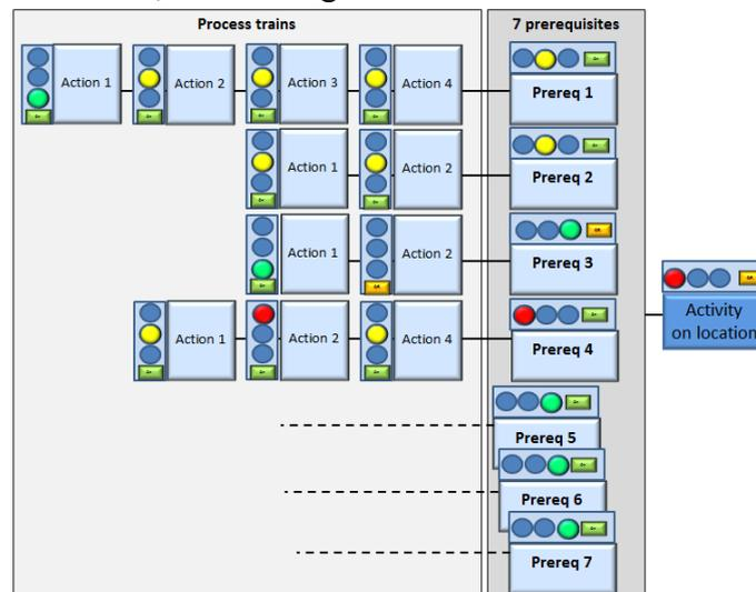
Figure 4: Status lights applied to process trains, seven prerequisites (visible on lookahead plan and production plans), and activity in the work breakdown structure
