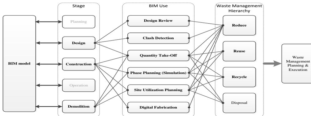
Figure 1. BIM-based Approaches to C&D Waste Management
