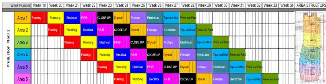
Figure 2: Increased concurrency of trades to eliminate WIP and reduce duration
