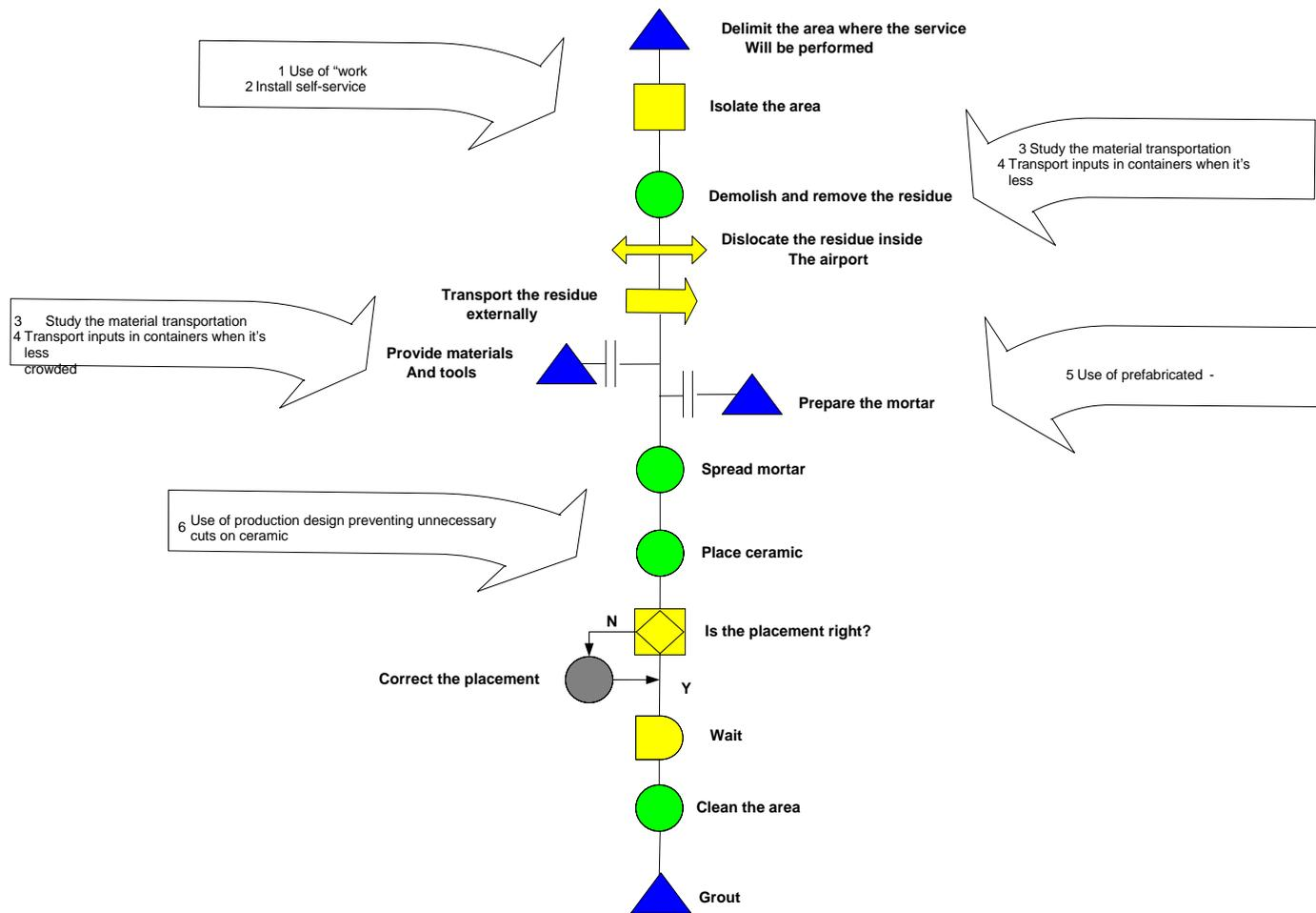
Figure 2: Flowchart of the replacement of ceramic coating in the construction process
