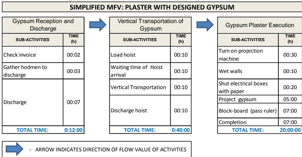
Chart 4 – Comparison between execution processes of plaster to each 5 m<sup>3</sup> of material and 1 cm of thickness to designed gypsum.
