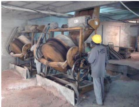
Concrete-mixer that produces the pre plaster at the construction site.
