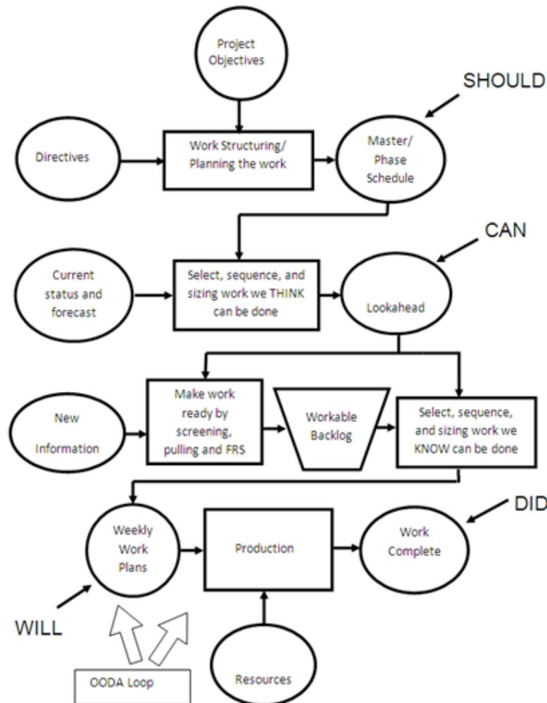
Figure 2. Project and Production Management Under Lean Construction (LCI 2001)
