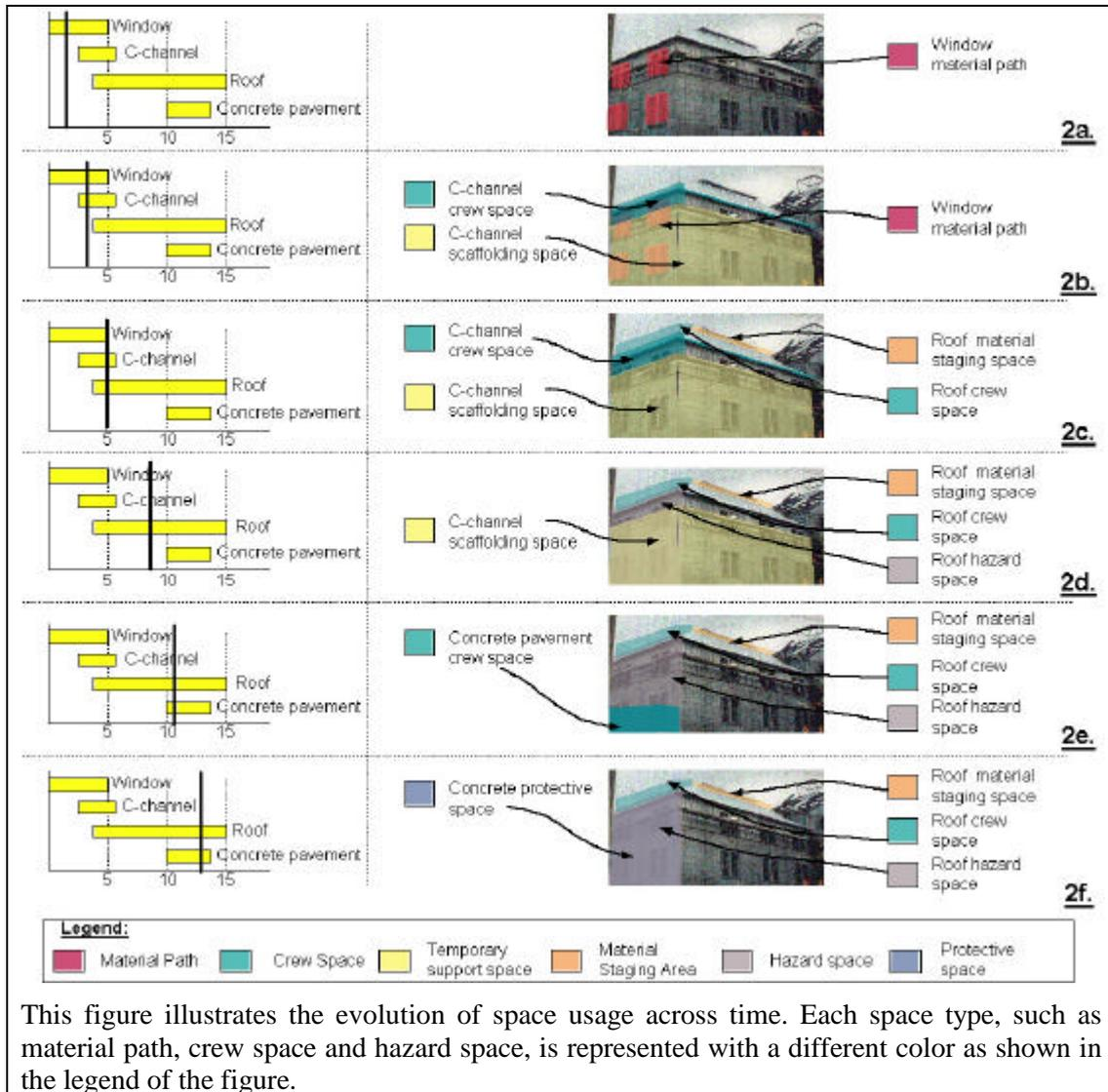
This figure illustrates the evolution of space usage across time. Each space type, such as material path, crew space and hazard space, is represented with a different color as shown in the legend of the figure.
