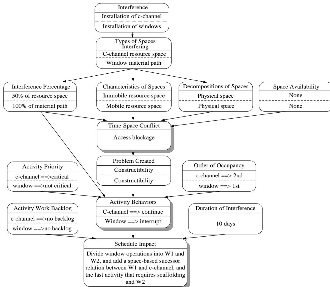
Figure 6: Application of the initial time-space conflict analysis framework for conflict between c-channel and window installation in the sample case
