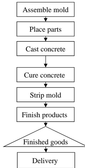
Figure 1: Precast production process
