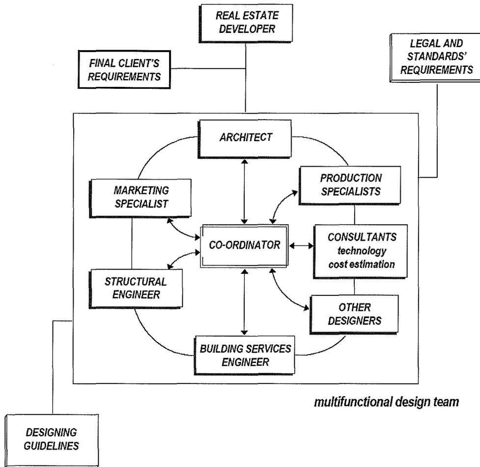
Figure 2: Proposal for a multi-functional 'design for production' team (Melhado 1994)
