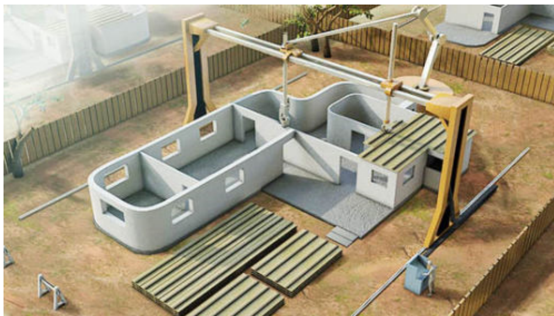
Figure 1: The Contour Crafting Machine ( www.contourcrafting.org )
