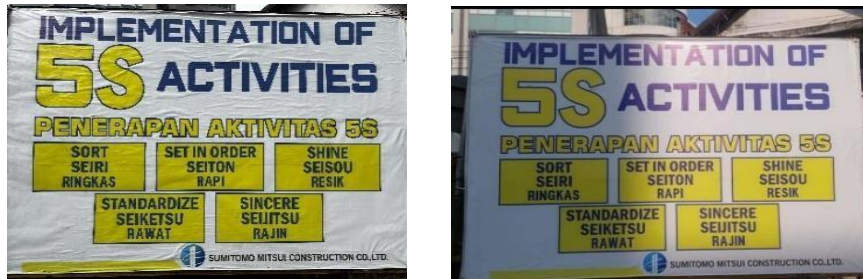
Figure 4: 5S Visual Management Awareness Installed at both Glodok and Kota Station
